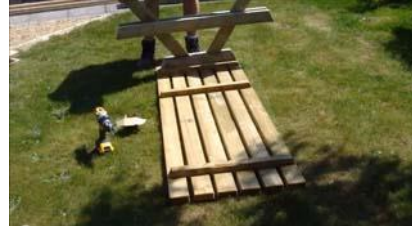
Place A-frame trestle into position
