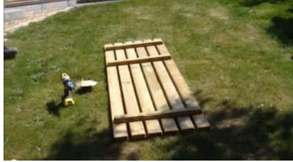
Put table-top face down on a flat surface
