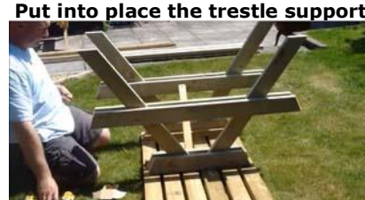
Place next A-frame trestle into position
